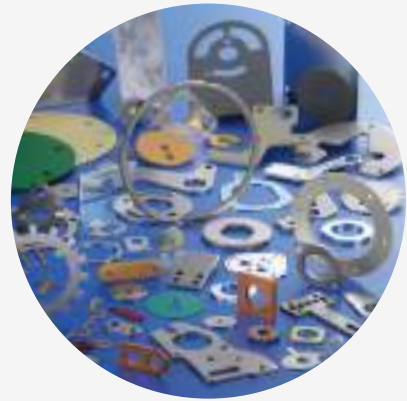
Flat blanking and piercing up to 12" by 12"
