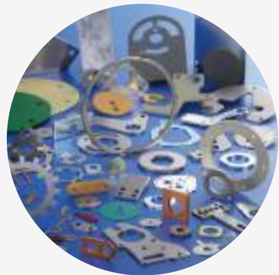
Flat blanking and piercing up to 12" by 12"
